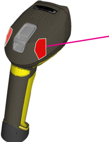
blinking red status indicator indicates low battery
